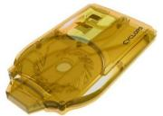
This patent-protected DPI can be produced cost-effectively because of its simple yet sophisticated design. Upon inhalation it uses the patient's breath to disperse the dry powder into small particles appropriately sized for deep lung deposition and, if required, rapid absorption of the drug into the circulation. Cyclops<sup>®</sup> has several advantages over standard-of-care products across key therapeutic areas. The above-mentioned attributes enable its **easy, hygienic**
