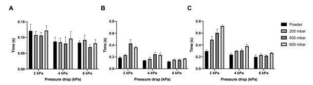
**Figure 7.** The dispersion times for 55 mg isoniazid. Panel (**A**) shows the time it took to empty the SDC, panel (**B**) shows the time it took for the bulk of the powder to be dispersed, and panel (**C**) shows the time needed to disperse the complete dose (average  $\pm$  SD, n = 5).
