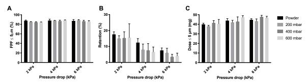
**Figure 8.** The effect of vacuum pressure on the dispersion of 57 mg amikacin. Panel (**A**) shows the FPFs found for the loose powder and three different pellets, panel (**B**) shows the inhaler powder retention, and panel (**C**) shows the FPD (average  $\pm$  SD, n = 5). The FPD is calculated by multiplying the FPF with the emitted dose (= FPF × (1 – retention)).
