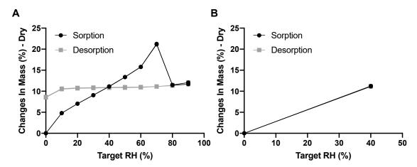
**Figure 2.** The DVS results for the amikacin formulation—panel (**A**) shows the sorption and desorption data from 0% to 90% RH and back in steps of 10% RH; panel (**B**) shows the data from 0% to 40% RH and back in steps of 40% RH (n = 2, both replicates shown).
