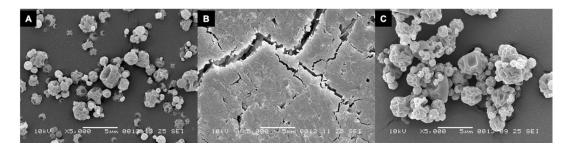
**Figure 4.** SEM images of the spray-dried amikacin formulation containing 1% L-leucine. Panel (**A**) shows the powder before DVS measurement. Panel (**B**) shows the same formulation after being exposed to 90% RH and panel (**C**) shows the same powder after being exposed to 40% RH during the DVS measurements. Magnification 5000× times.
