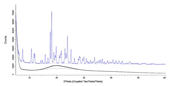
**Figure 5.** The X-ray spectra of the amikacin 1% L-leucine samples. The black line is the amikacin sample stored at 0% RH and the blue line is an amikacin sample stored at 80% RH for one week and is offset by 10,000 counts.
