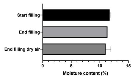
**Figure 3.** The moisture contents for the amikacin formulation automatically filled into SDCs. Start filling samples are the first five SDCs filled under normal conditions. End filling samples are the last five SDCs filled under normal conditions. The end filling dry air samples are the last five SDCs filled when automatic filling took place under dry air (average  $\pm$  SD, n = 10).
