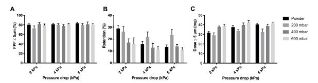
**Figure 6.** The effect of vacuum pressure on the dispersion from the Cyclops<sup>®</sup> inhaler of 55 mg isoniazid. Panel (**A**) shows the FPFs for the loose powder and the three different pellets, panel (**B**) shows the retention, and panel (**C**) shows the FPD (average  $\pm$  SD, n = 5). The FPD is calculated by multiplying the FPF with the emitted dose (= FPF × (1 – retention)).
