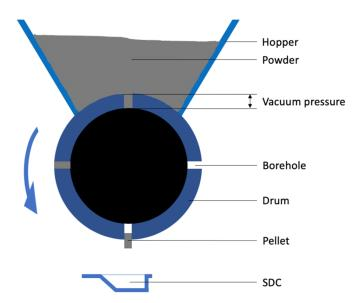
Figure 1. A schematic representation of the vacuum drum filler used in this study.
