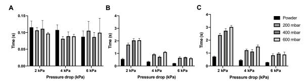
**Figure 9.** The dispersion times for 57 mg amikacin. Panel (**A**) shows the time it took to empty the SDC, panel (**B**) shows the time it took for the bulk of the powder to be dispersed, and panel (**C**) shows the time needed to disperse the complete dose (average  $\pm$  SD, n = 5).
