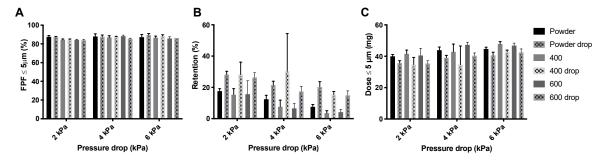
**Figure 11.** Effect of the drop test on the dispersion of 57 mg amikacin by the Cyclops<sup>®</sup>. Panel (**A**) shows the FPF of the different products before and after the drop test, panel (**B**) shows the retention and panel (**C**) shows the FPD (average  $\pm$  SD, n = 5). The FPD is calculated by multiplying the FPF with the emitted dose (= FPF × (1 – retention)).
